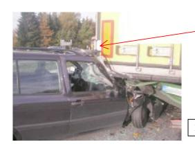
GRSG-104-49 (FIA-page  $6-2^{\rm nd}$  top figure). Hinges and latches are located higher than the starting point of under-run, thus the risk of injury due to hinges an to the passenger cars' drivers and/or passengers is low.
