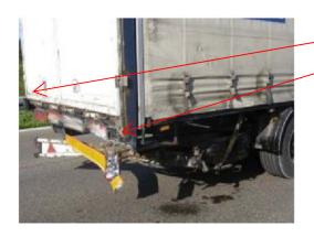
GRSG-104-49 (FIA-page 6 -bottom right figure). Rubber on the right hand side is delaminated, crushed by the passenger car impact.
