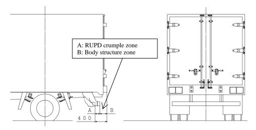
Concerning tail lamps and rubbers, they are not as strong as the passenger cars structure and will be detached by a rear end collision:
