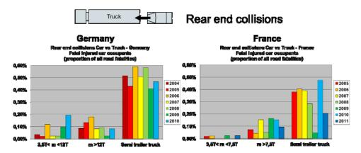
A detailed analysis of all rear end collisions between trucks/trailers and cars based on German accident data show that in more than 85% with fatal injured car occupants a semi-trailer truck was involved (see following table).
