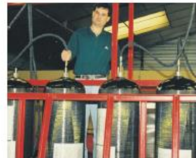
HYDRAULIC TEST PRESSURE 300 BAR
