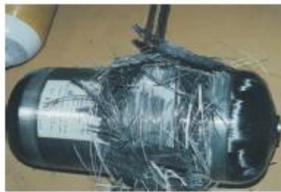
HYDRAULIC BURST TEST
