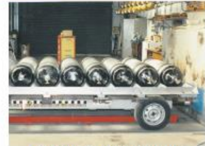
FRONTAL CRASH TEST 30 G FOR BUS
