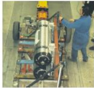
FRONTAL CRASH-TEST 30G FOR TRUCKS
