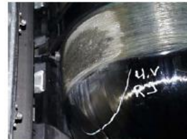
Mixed UV and chemical damages
