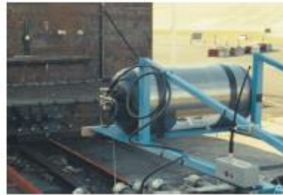
CATAPULT LAUNCHING AT 50 KM/H against a metallic sharp edge
