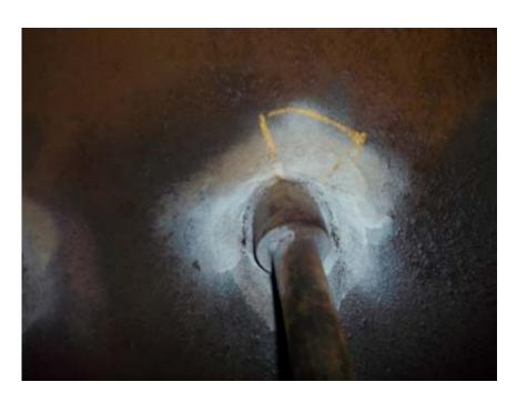
Nozzle 1 houses the temperature gauge blind pocket and has a 25 mm long crack as indicated below:
