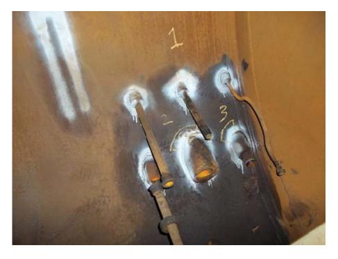
Following the initial indications of cracking light grinding of the surface was undertaken to ensure that it was not just weld overlap, however it was confirmed that all three were hairline cracks (the white background paint and black indicator has now made these very visible to the naked eye).
