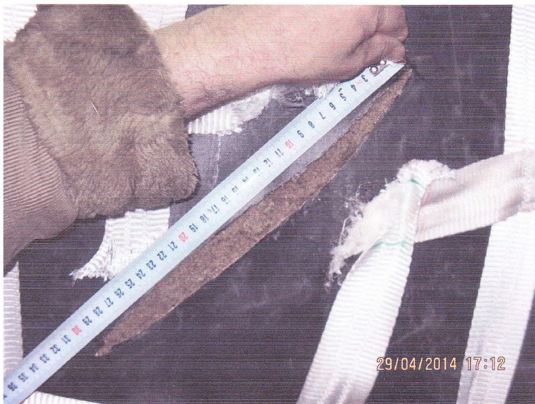
Fig. 6.2 Container after tear testing
