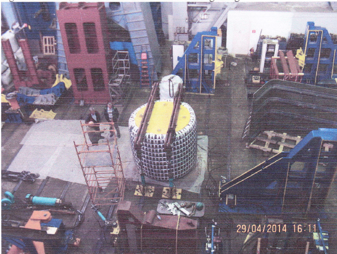
Fig. 5.3. Container on test bench after stacking test (top view) beginning
