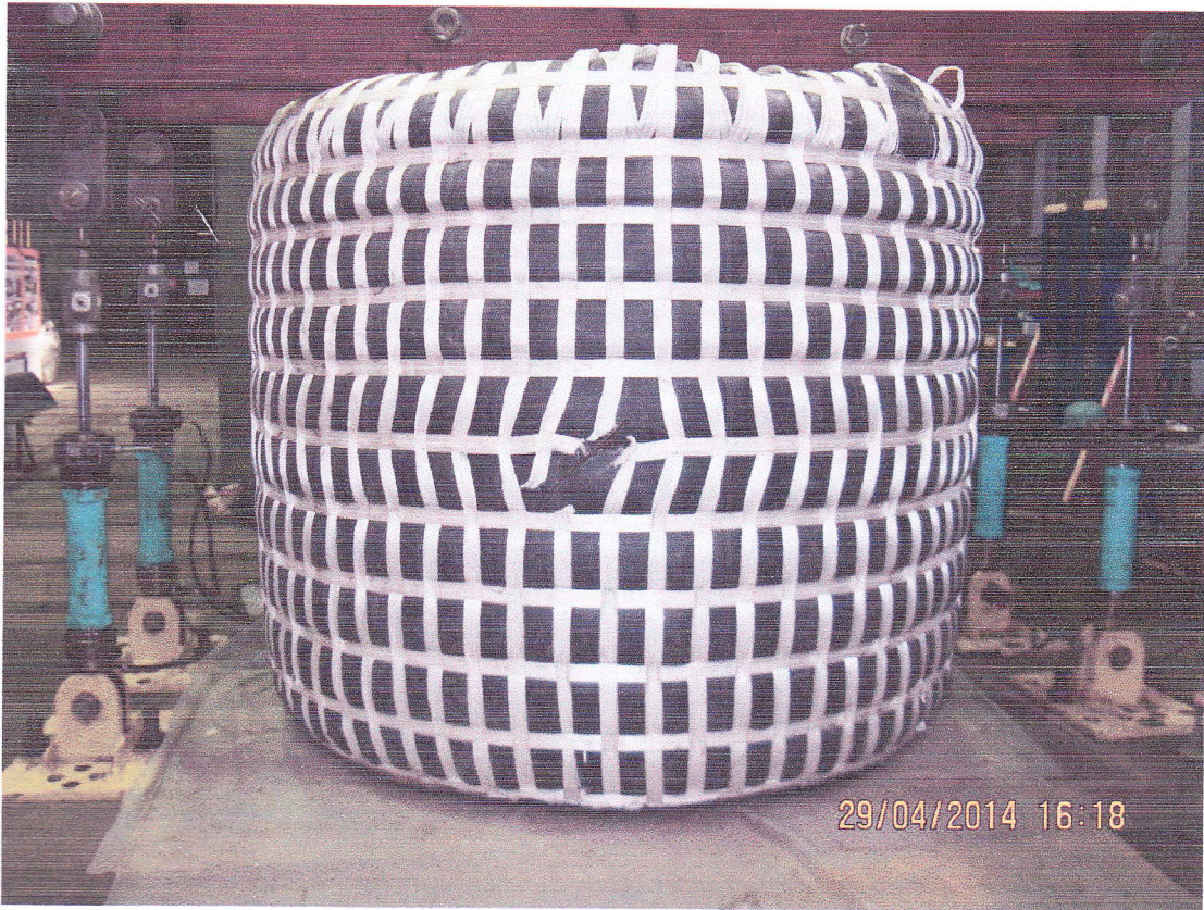
Fig. 6.1 Container under load 28 tf before tear testing
