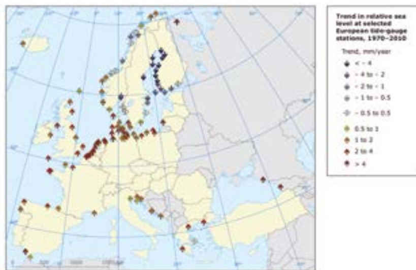
Figure 5 Trends (1970-2010) in relative sea level at selected European tide gauge stations (not corrected for local land movement) (from EEA (2012), see also HTTP://WWW.PSMSL.ORG/PRODUCTS/TRENDS/ ).
