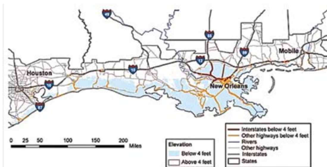
Figure 23 Roads at risk in the event of a sea level rise of about 1.2 m (4 feet), which is within the range of projections for this part of the United States of America Gulf Coast in this century under medium- and high-emissions scenarios. In this case, 2,400 miles of major roads are predicted to be inundated (CCSP, 2008; Karl et al., 2009).
