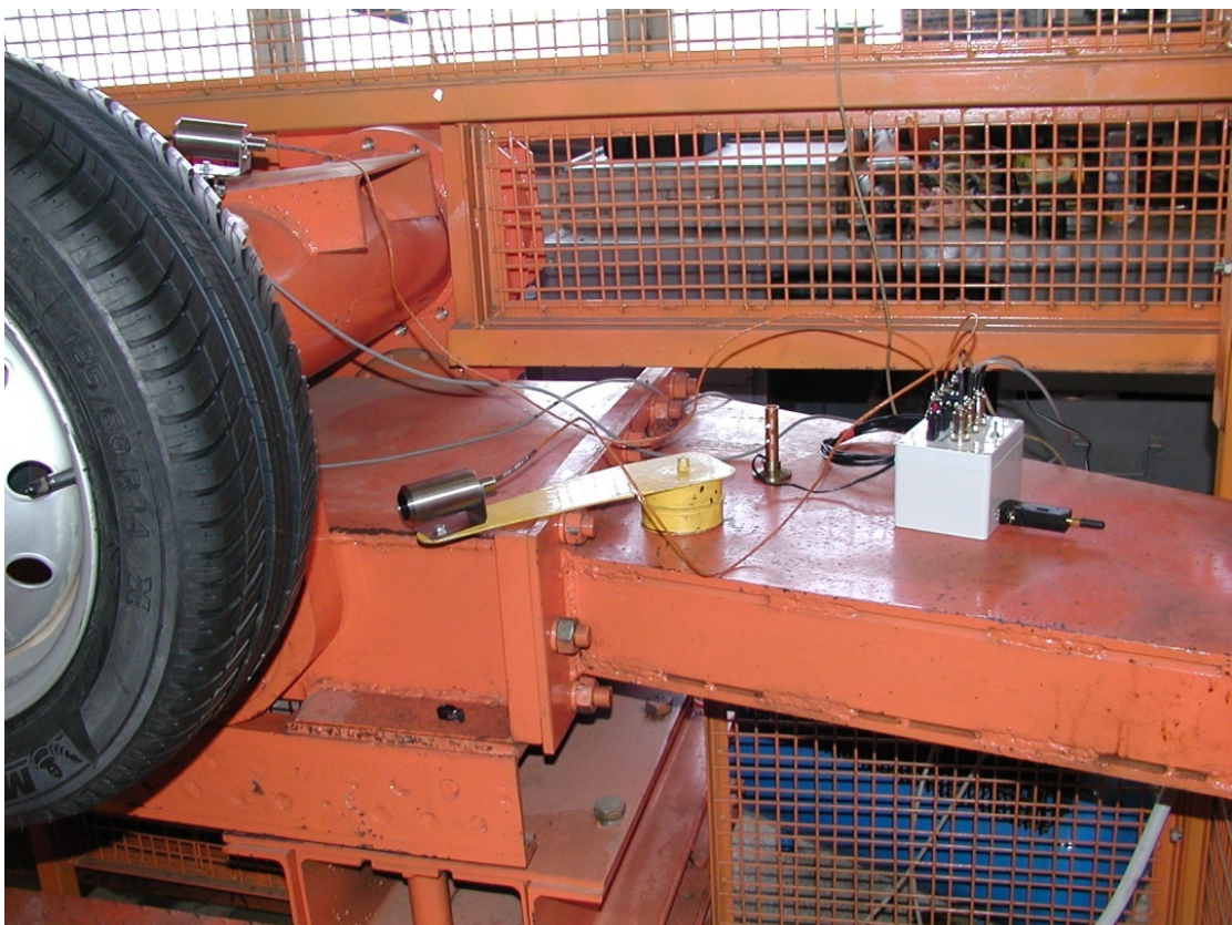
Figure 8. NAMI-354 test machine (at the top) with device NAMI-357 (bottom). “C” – electromagnetic clutch which decouples drum from motor during coastdown.
