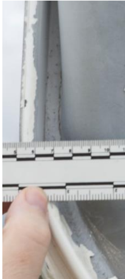
2011 - crack at the toe of the fillet weld between the front end dish and extrusion band at the bottom of the impact area
