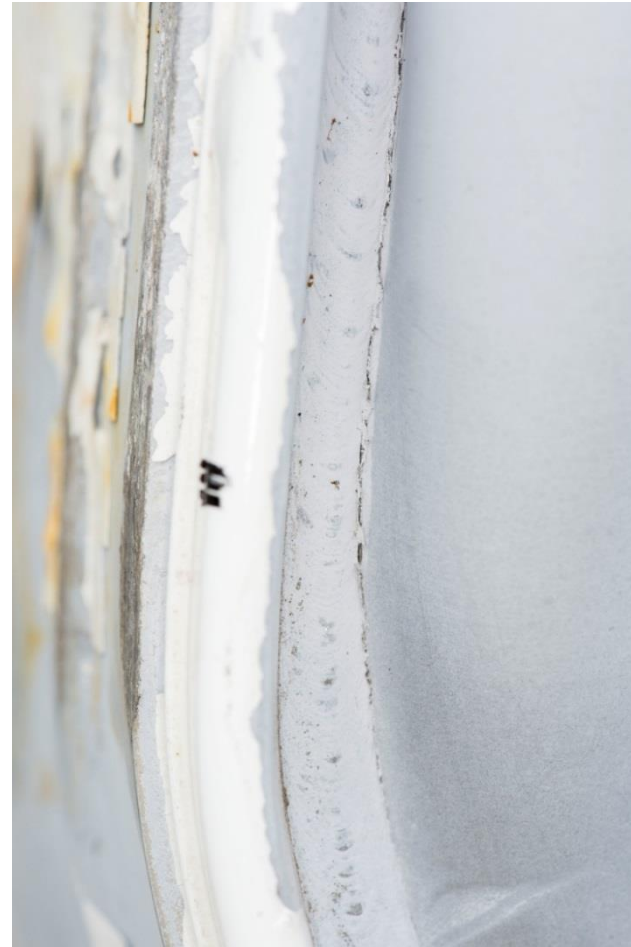
2011 - crack at the toe of the fillet weld between the front end dish and extrusion band at the bottom of the impact area
