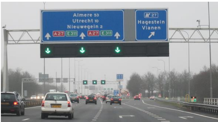
FIGURE 7. CONTRADICTORY AND UNNECESSARY USE OF OPPOSING ARROWS FOR INDICATING DIRECTIONS AHEAD
