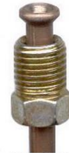
A1 3/8 x 24 UNF common American nut with 45 degree double flare on 3/16"/4.75MM dia. tube
