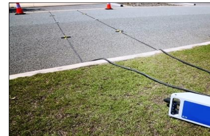
Short Duration (Portable) Traffic Counter & Classifier
