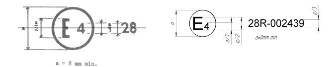
The above approval mark affixed to a vehicle indicates that, pursuant to Regulation No. 28, this vehicle type has been approved in the Netherlands (E 4), with regard to its audible signals. The first two digits of the approval number indicate that Regulation No. 28 was in its original form.
