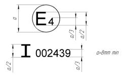
The above approval mark affixed to an audible warning device shows that this audible warning device of Class I has been approved in the Netherlands (E 4) under approval number 002439. The first two digits of the approval number indicate that the approval was granted in accordance with the requirements of Regulation No. 28 in its original form.
