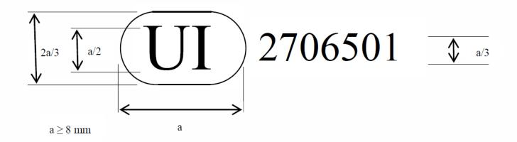
The above Unique Identifier marked on the device shows that the type concerned has been approved and that the relevant information on that type approval can be accessed on the UN secure internet database by using 2706501 as the Unique Identifier.
