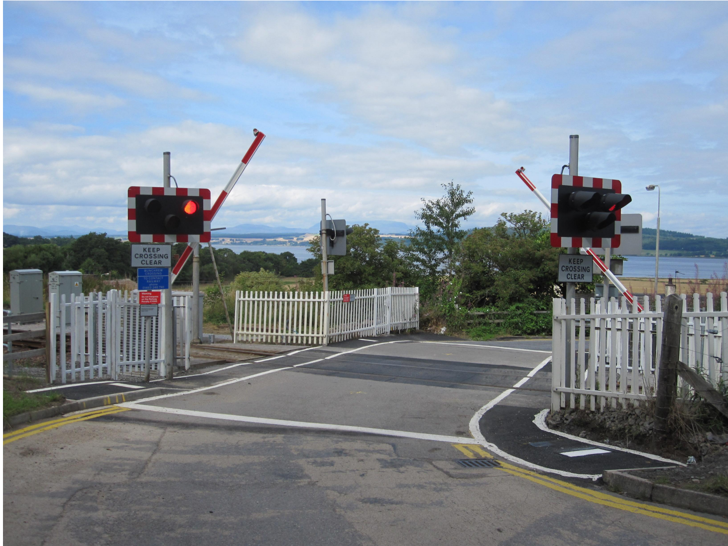
Courtesy of © G. Wallace, Bunchrew Level Crossing with Automatic Half Barriers, Scotland, 2013.
