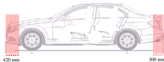
Figure 25 Prohibited installation positions (red) for vehicle independent approved REESS
