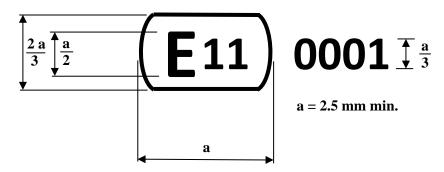
The above approval mark affixed to a gas-discharge light source indicates that the light source has been approved in the United Kingdom (E 11) under the approval code 0001."
