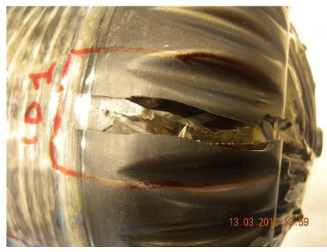
At the opening of the box after 1 year of storage (6 broken over 12 cylinders)
