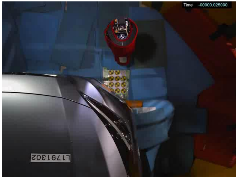
Firing signal of the pedestrian airbag
