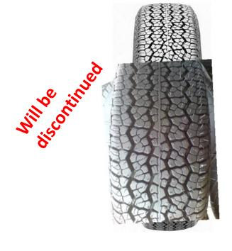
Must be used as **reference tyre** to determine the relative wet grip performance of the candidate tyre It **can be** used to verify / certify track friction properties (one of the 2 possible methods)
