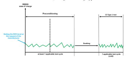
1.3. Test sequence OVC-HEVs and OVC-FCHVs\_according to option 3
