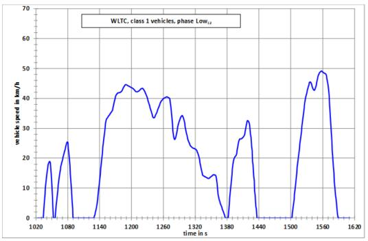
$Table \ A1/1 \\ WLTC, Class \ 1 \ cycle, phase \ Low_{11} \ (Second \ 589 \ is \ the \ end \ of \ phase \ Low_{11} \ and \ the \ start \ of \ phase \ Medium_1)$
