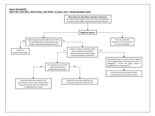
4. PEVs equipped with a driver-selectable mode
