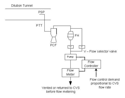
Figure A5/13 **Double dilution particulate sampling system**
