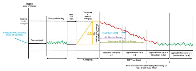
1.2. Test sequence OVC-HEVs according to Option 2
