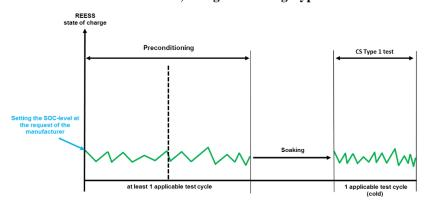
1.3. Test sequence OVC-HEVs and OVC-FCHVs\_according to option 3
