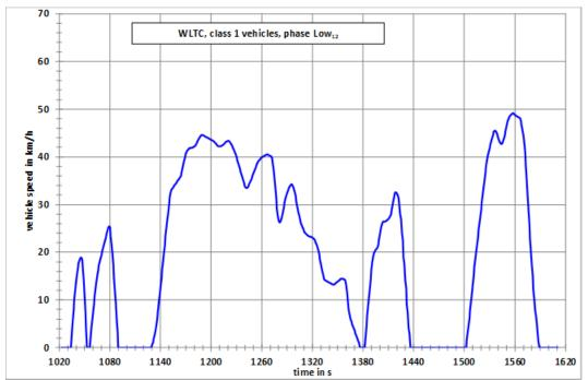
$Table \ A1/1 \\ WLTC, Class \ 1 \ cycle, phase \ Low_{11} \ (Second \ 589 \ is \ the \ end \ of \ phase \ Low_{11} \ and \ the \ start \ of \ phase \ Medium_1)$
