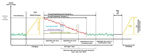
1.2. Test sequence OVC-HEVs and OVC-FCHVs\_according to option 2
