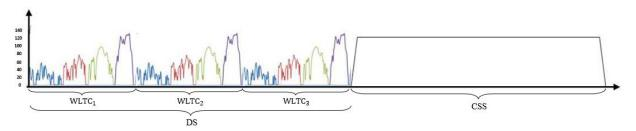
The dynamic segment DS is used to calculate the energy consumption of the phase considered, the applicable WLTP city cycle and the applicable WLTP test cycle.
