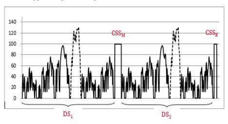
The dynamic segments  $DS_1$  and  $DS_2$  are used to calculate the energy consumption of the phase considered, the applicable WLTP city cycle and the applicable WLTP test cycle.
