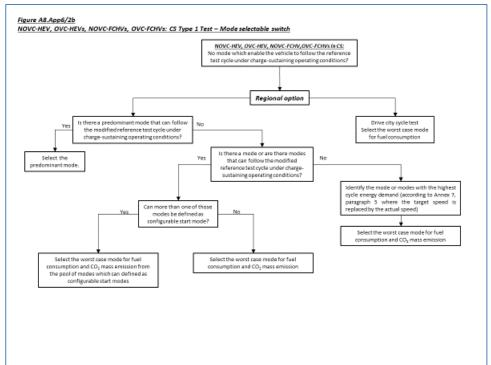
4. PEVs equipped with a driver-selectable mode
