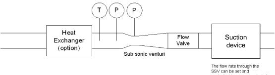
controlled by speed control of the flow and/or flow valve
