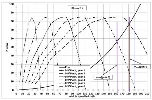
Figure A2/1b **An example where ng**<sub>vmax</sub> is the 2<sup>nd</sup> highest gear
