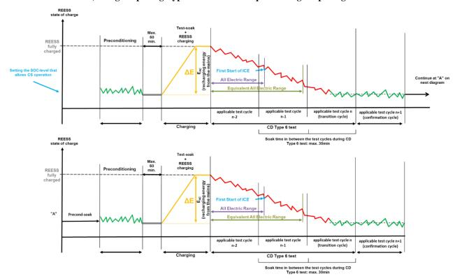
2. Test sequence NOVC-HEVs Charge-sustaining Type 6 test (Figure S-A1.App1/7)
