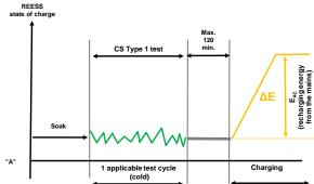
1.4. Test sequence OVC-HEVs and OVC-FCHVs\_according to option 4
