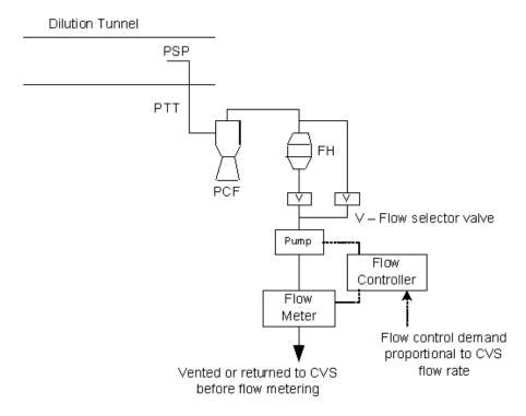
Figure A5/13 **Double dilution particulate sampling system**
