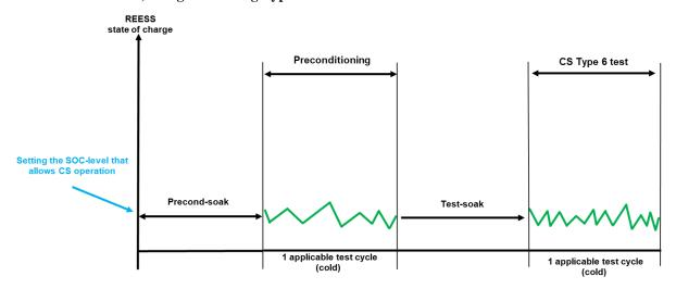
1.3. Test sequence OVC-HEVs according to Option 3
