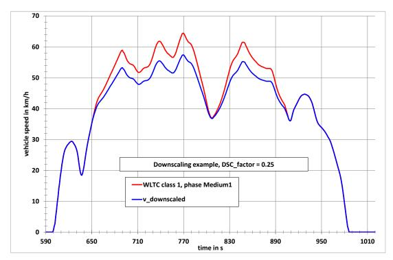
For the Class 1 cycle, the downscaling period is the time period between second 651 and second 906. Within this time period, the acceleration for the original cycle shall be calculated using the following equation:
