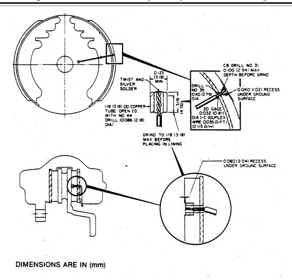
Figure 1-Typical Plug-Type Thermocouple Installations
