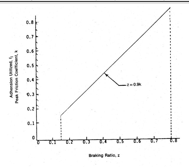
Figure 2-Adhesion Utilization Requirements
