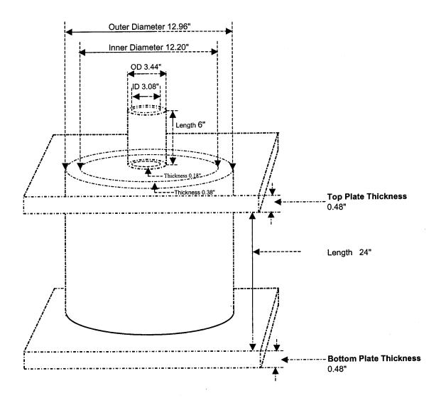
Material of the pipe: Schedule 40 c carbon (A53 Grade B) steel
