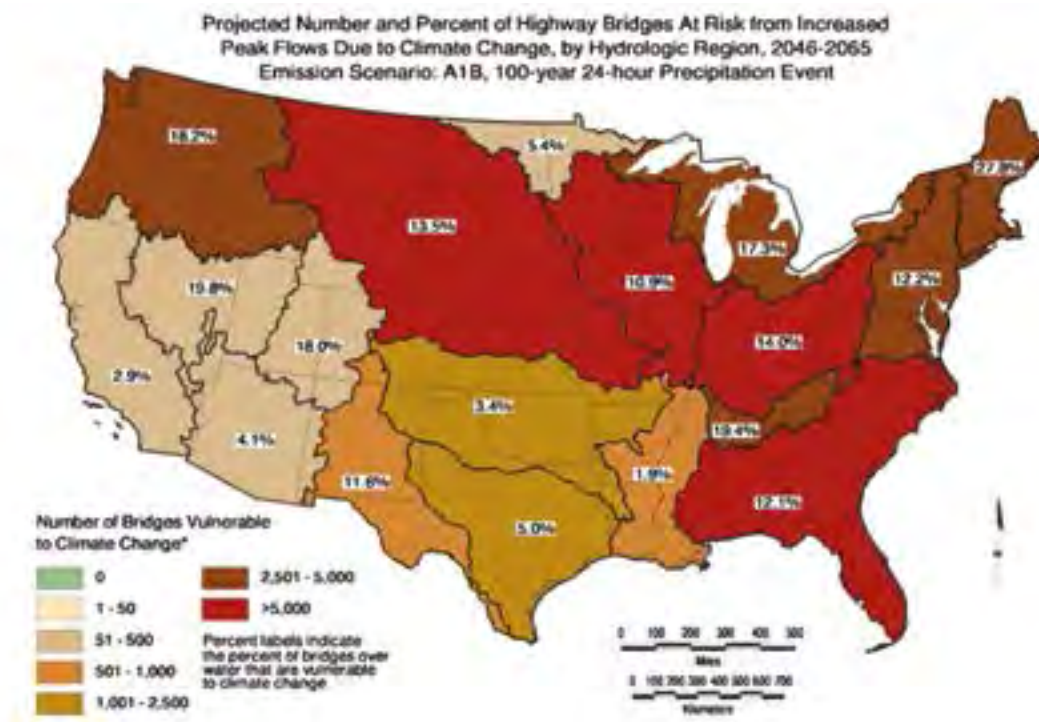
Figure 30 Distribution (projected number and percentage) of the United States of America highway bridges at risk from increased peak flows due to climate change (Emission Scenario A1B, 100-year event, 24-hour precipitation for the period 2046-2065 (Wright et al., 2012).
