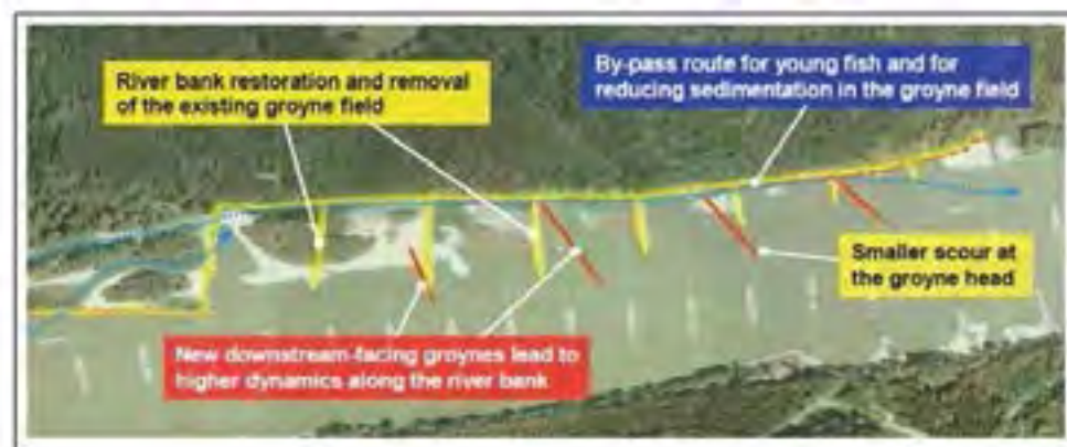
Figure 59 Adaptation river engineering methods used in Pilot Project Witzelsdorf (Siedl, 2012). The old groynes (yellow) were removed and replaced by new groynes of improved design to change favorably the river flow and sediment dynamics.
