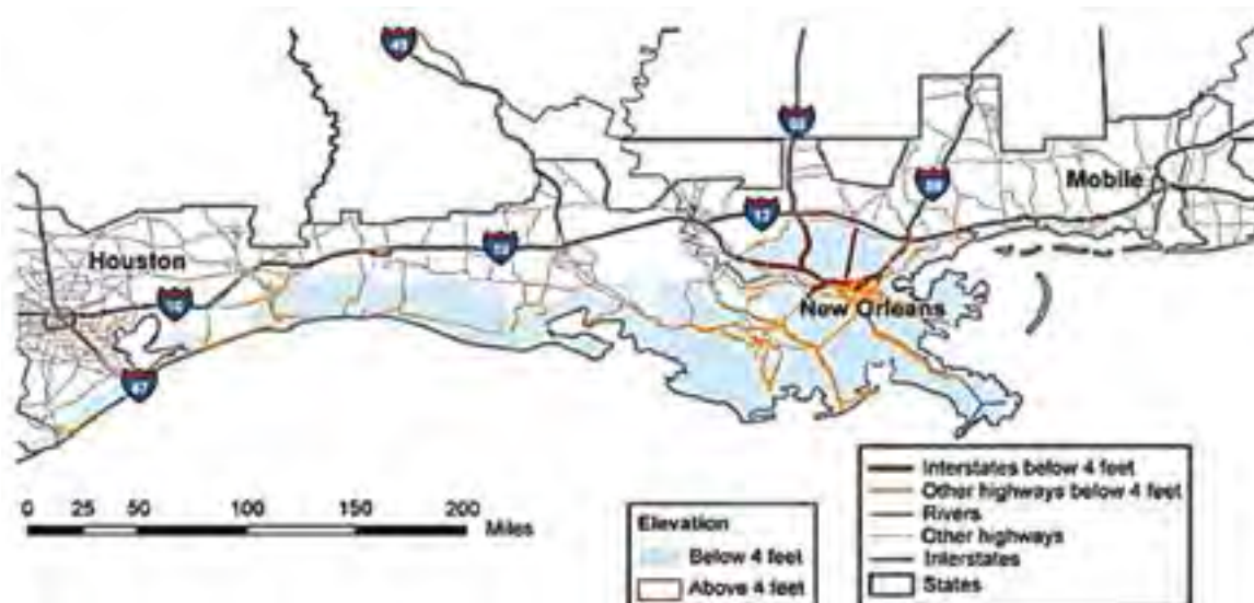
Figure 23 Roads at risk in the event of a sea level rise of about 1.2 m (4 feet), which is within the range of projections for this part of the United States of America Gulf Coast in this century under medium- and high-emissions scenarios. In this case, 2,400 miles of major roads are predicted to be inundated (CCSP, 2008; Karl et al., 2009).
