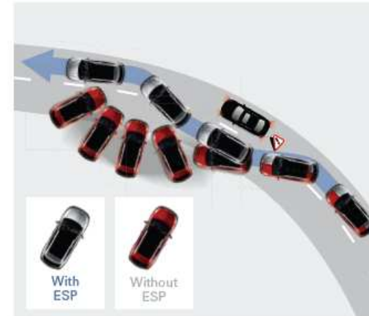
Optimum brake-force distribution under the critical situation.
