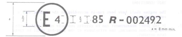
The above approval mark affixed to an engine shows that the engine type concerned has been approved in the Netherlands (E 4) with regard to the measurement of the net power, pursuant to Regulation No. 85 and under the approval number 002492. The approval number indicates that the approval was granted in accordance with the requirements of Regulation No. 85 in its original form.
