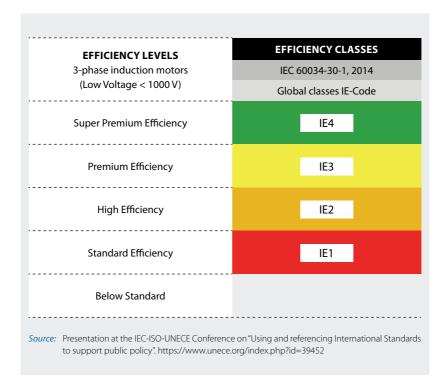
in detail: the IEC standards classify four classes with different levels of efficiency: the European Commission (EC) regulation stipulates the second highest class as mandatory for all new motors from 1 January 2015. In this way, the EC made ecodesign mandatory and promoted energy savings through incorporating international standards into regional regulation.
