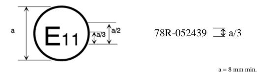
The above approval mark affixed to a vehicle<sup>1</sup> shows that the vehicle type concerned has, with regard to braking, been approved in the United Kingdom (E 11) pursuant to UN Regulation No. 78 under approval number 052439. The first two digits of the approval number indicate that UN Regulation No. 78 already included the 05 series of amendments when the approval was granted.
