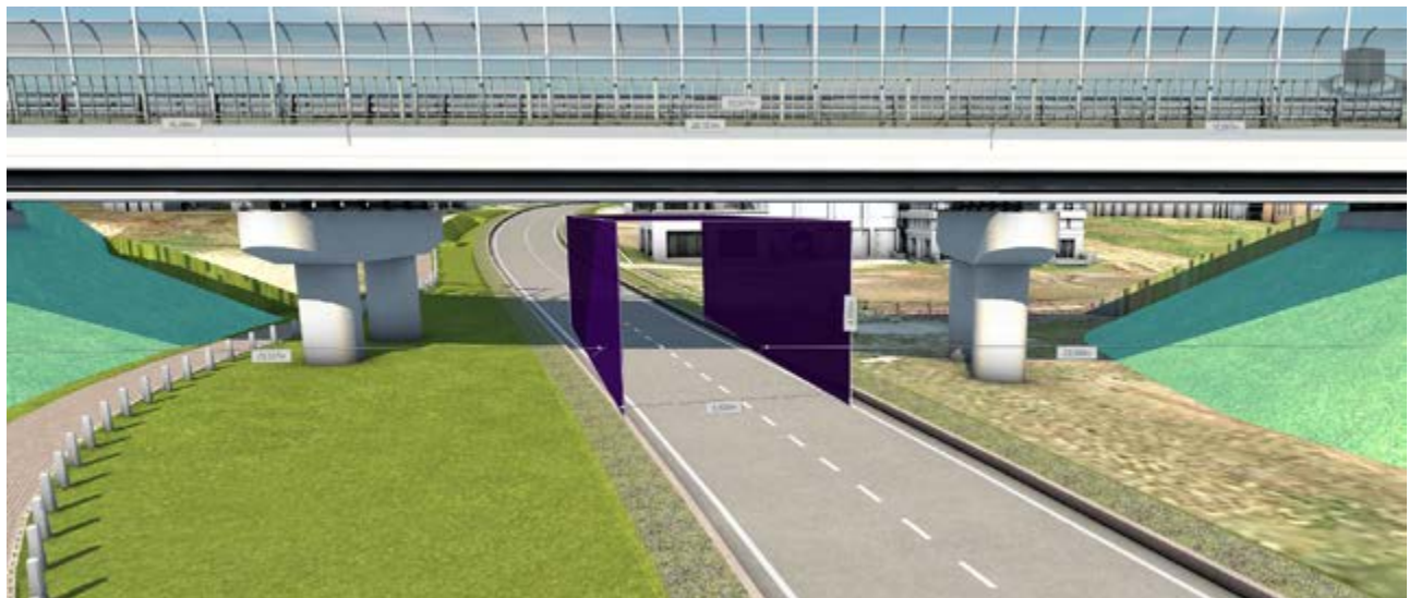
Figure 31 Clearance check of planned overpass
