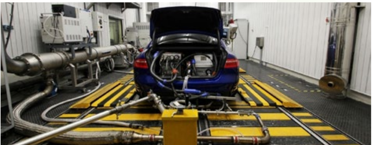
Testing emissions of a vehicle © IDIADA - Spain
