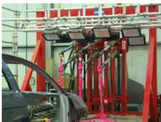
Testing machine for seat anchorages © INTA - Spain
