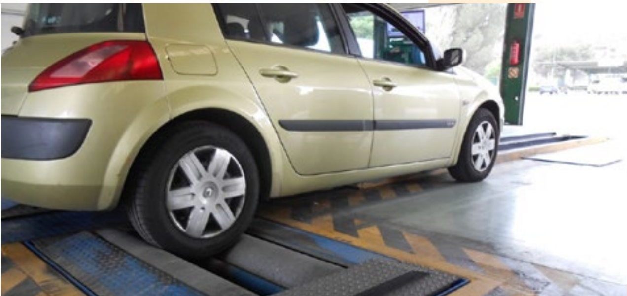
Testing braking efficiency © EuroMed - TSP
