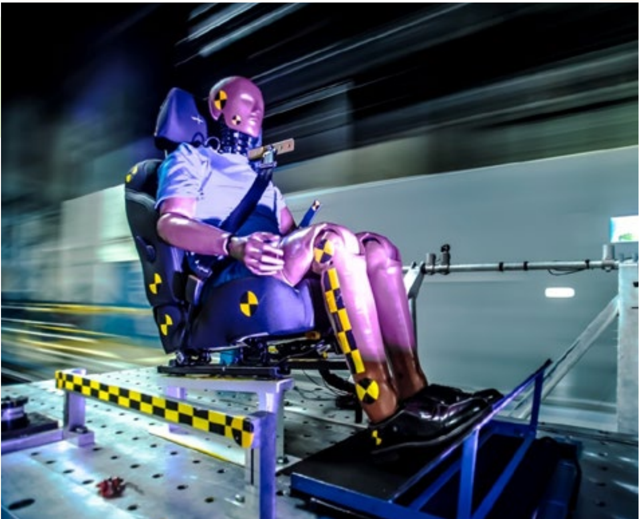
Inverse Catapult for testing safety belts © UTAC CERAM - France
