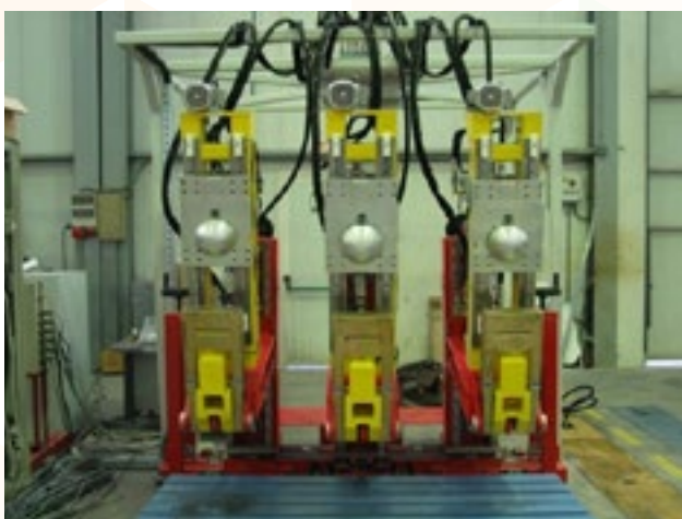
Testing machine for safety belt anchorages © INTA- Spain
