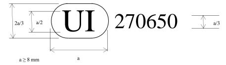
The above Unique Identifier shows that the type concerned has been approved and that the relevant information on that type-approval can be accessed on the UN secure internet database by using 270650 as Unique Identifier. Any leading zeroes in the Unique Identifier may be omitted in the approval marking.
