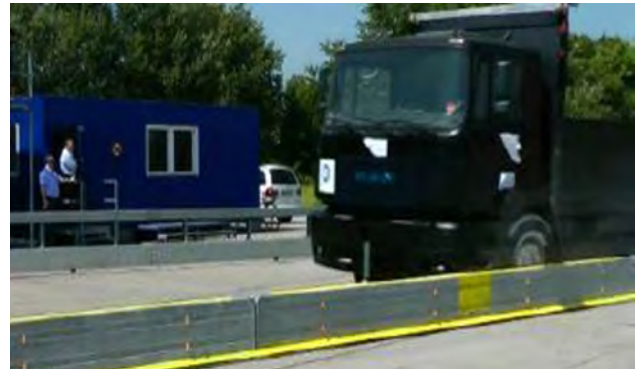
Figure 10: Slim temporary safety barrier
