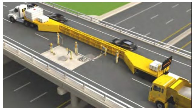
Figure 12: Truck-mounted mobile barrier system
