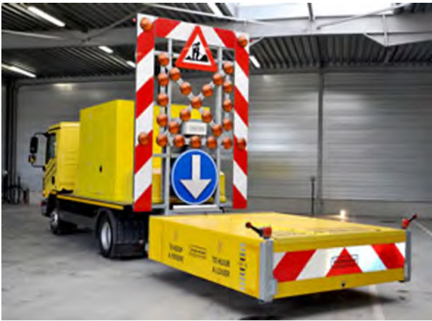
Figure 15: Example of a truck mounted attenuator
