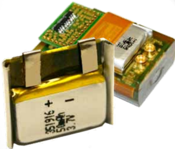
External fixed Backup Battery with status monitoring by software.
