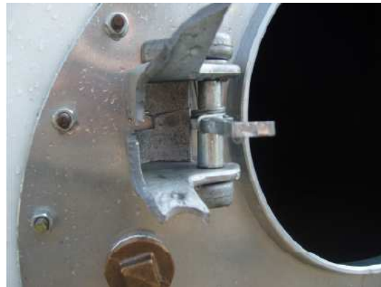
Picture 4: Broken locking device after the test
