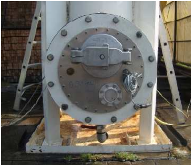
Picture 2: Dome cover manufactured in an ADR member state fitted to the test apparatus
