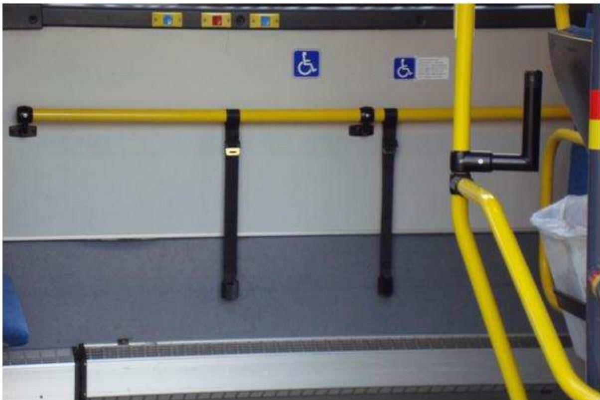
Straps for the stability of trams on the tram and wheelchair space
